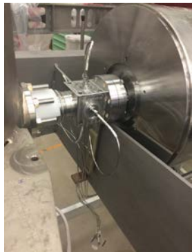
Cold beam- position monitor
