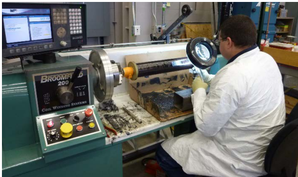
Superconducting magnet fabrication
